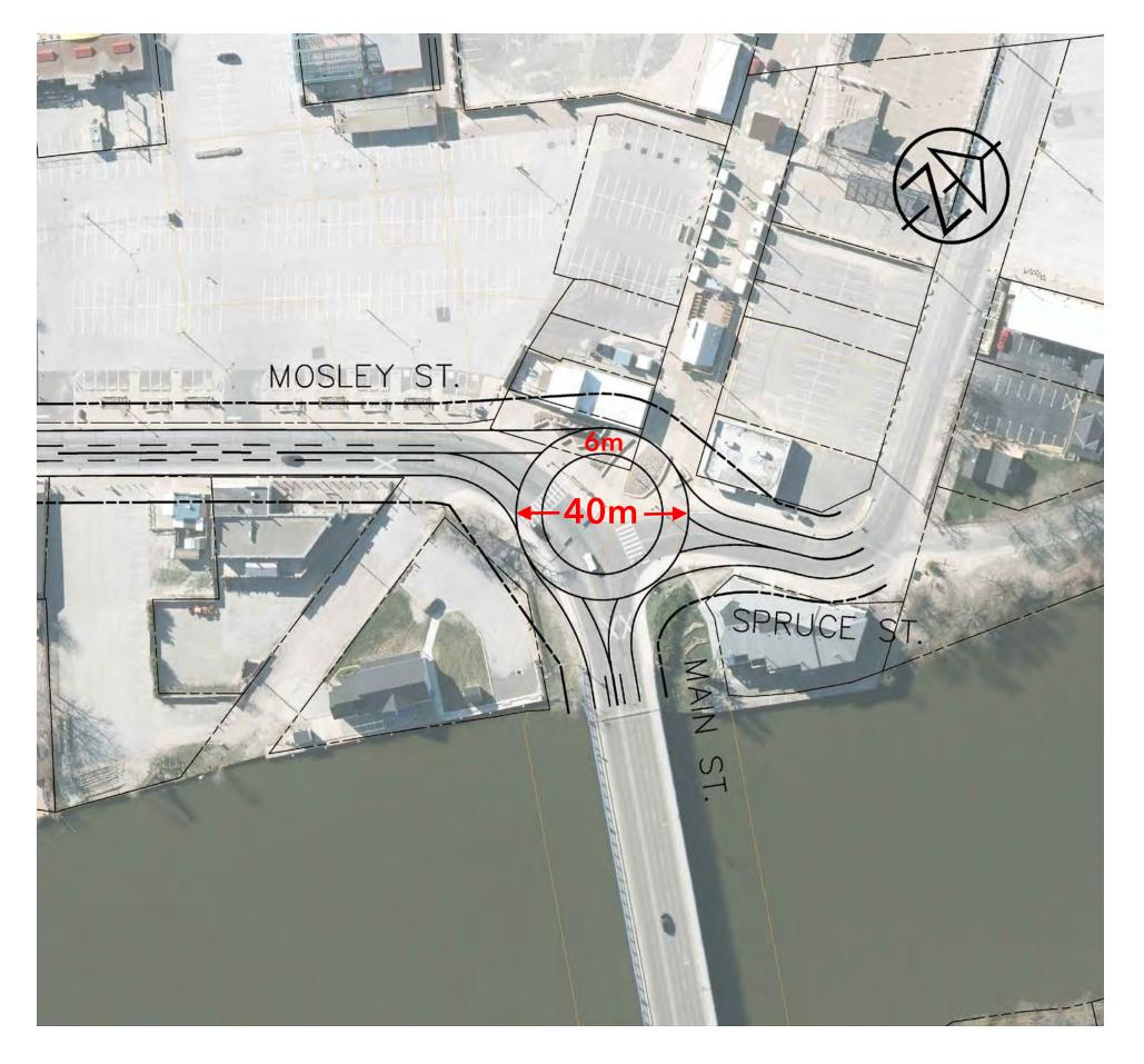
Roundabout configurations are PRELIMINARY in nature and are only intended to show the overall design approach, roundabout footprint and potential property impacts. Further detail design will be required.
